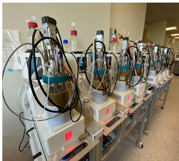
Bioprocess for PHA bioplastic production
