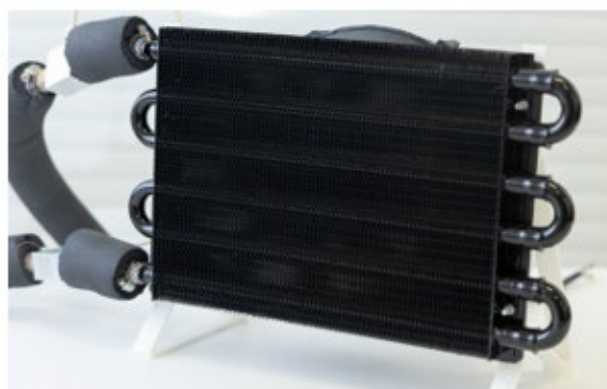
Experimental Heat Sink coated in graphene
