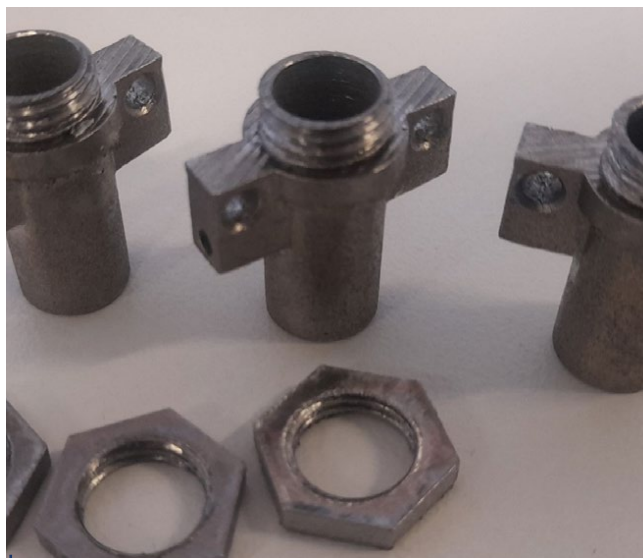
Probe holders and flange nuts 3D printed in IN625
