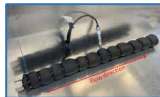
Detachable Test Section (0.83" ID)
